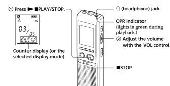
After playing back one message, the unit stops at the beginning of the next message. When the continuous play function is set to "ON" (see the reverse side), the unit stops after playing all messages in a folder. When the last message on a folder has been played back, the unit stops at the beginning of the last message.
